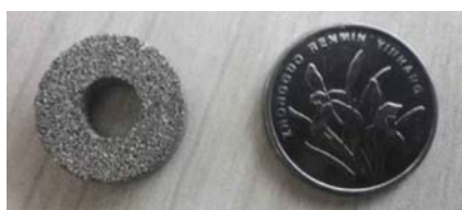
Fig. 1 Annular sintered metal powder porous media
